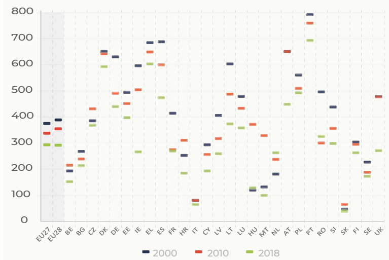
Electricity production footprint by Member State for 2000 2010 and 2018 in gCO 2 eq/kWh of electricity
